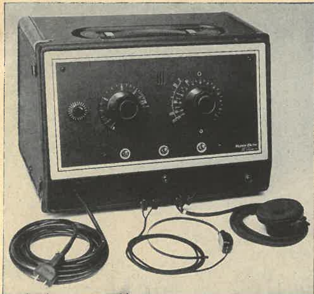
Fig. 1. A portable audiometer with bone conduction receiver at center and air conduction receiver at right. The small knob at left is for calibration. The large knobs are for frequency and intensity. (Courtesy Bell Telephone Laboratories)
